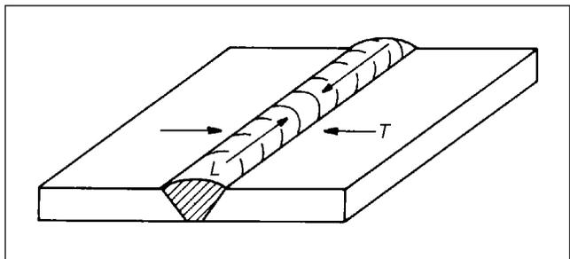
**Figure 7.1—Longitudinal (L) and Transverse (T) Shrinkage Stress in a Butt Joint Weld**
